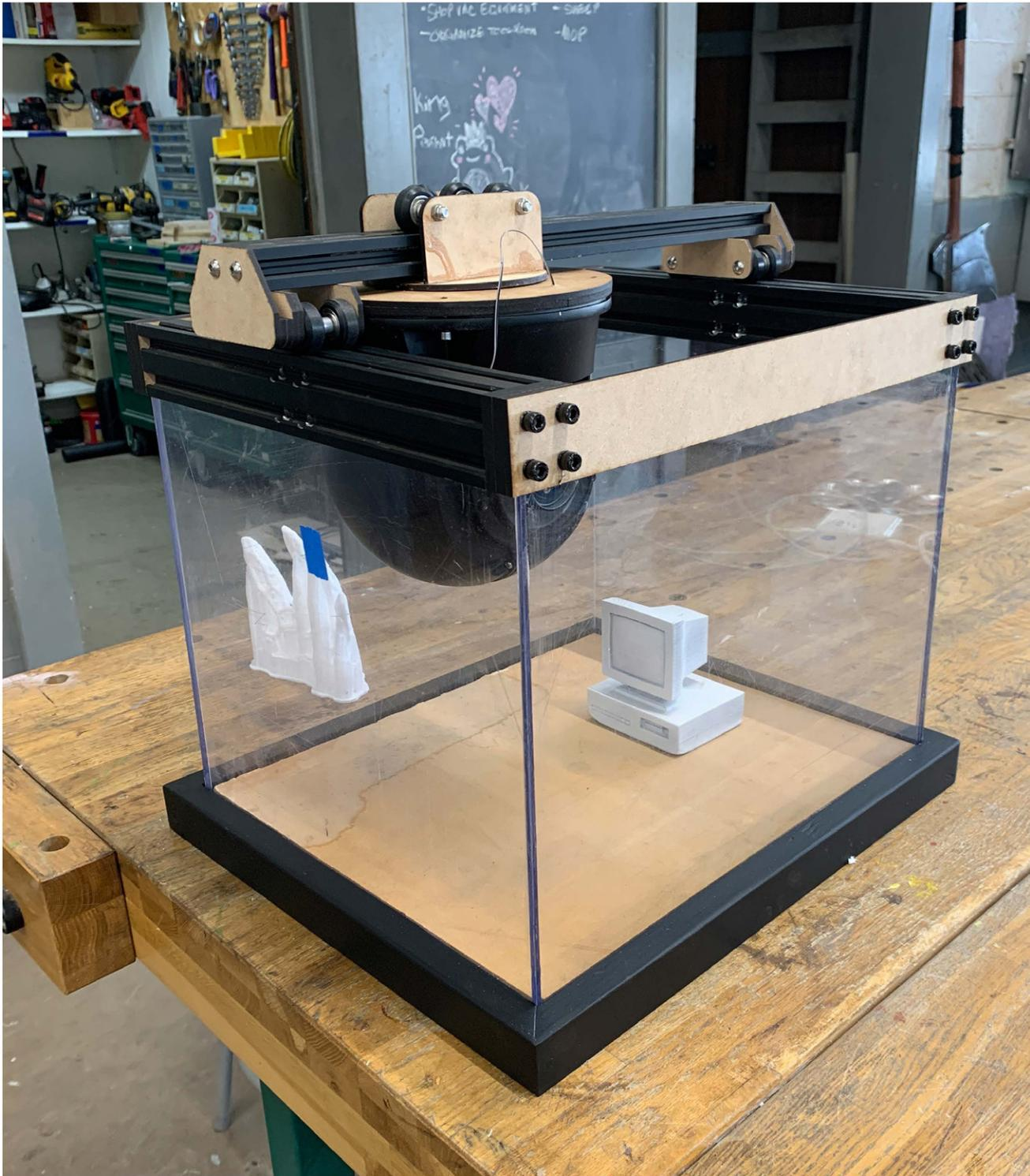
This is the first progress photo of the project. I had quickly build a carriage system for the camera. This allows it to move freely in the enclosure.
