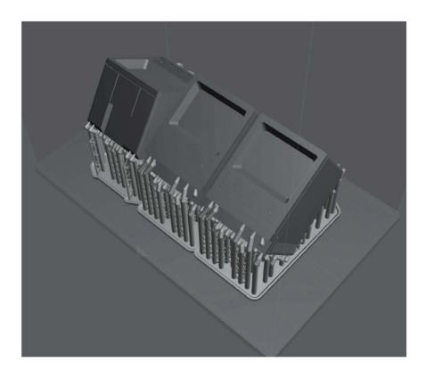
All of these photos are of screen-shots of the model, supports, and rafts built in Lychee Slicer. These were exported into g-code for the resin printer.
