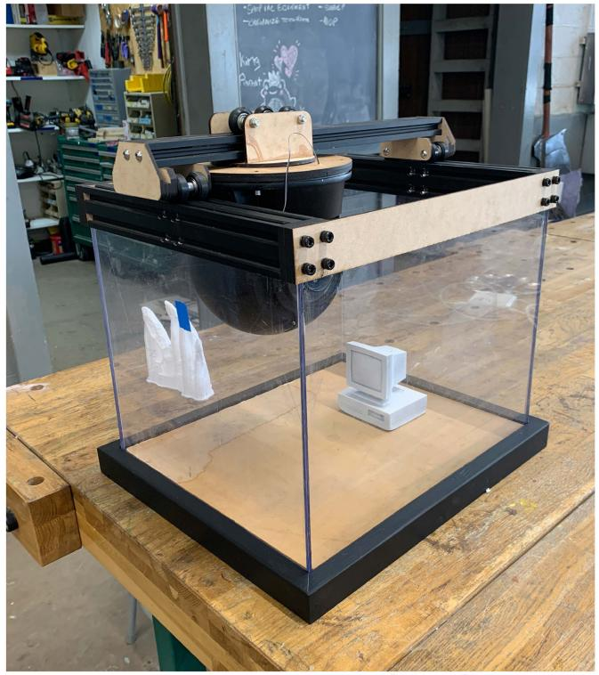
This is the first progress photo of the project. I had quickly build a carriage system for the camera. This allows it to move freely in the enclosure.
